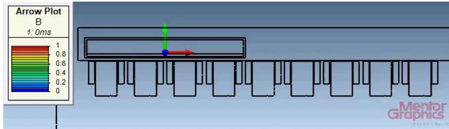
This video shows the vehicle launch from a different viewpoint. The simulation covers the first few tenths of a second after the power is switched on. The oscillating behavior is typical of this type of MagLev, and is one of the reasons why this type has not seen widespread use. In fact, the vehicle in this example is too short to be very stable around the pitch axis and it can be seen that the lower rear edge strikes the track. The arrow plot shows the magnetic field around the vehicle.
